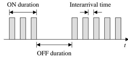
Fig. 4. ON/OFF traffic model.
